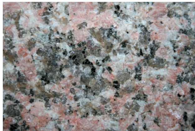
FIGURE 1-2 Interlocking grains in granite. The pink and white grains are two kinds of feldspar, the gray grains are quartz, and the black grains are mafic minerals. The smaller quartz grains are the size of grains of sand. (Sabena Jane Blackbird/Alamy.)
